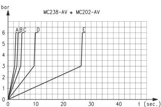
Pressurisation times as to the n° of turns of the regulation screw, with downstream volume of 5 litres. A = 5 turns - B = 4 turns - C = 3 turns - D = 2 turns - E = 1 turn. "K" = n° of turns of the regulation screw required to obtain the required pressurisation time with an inlet pressure of 6 bar. Variations of the inlet pressure can cause deviations of the pressure time by  $\pm$  20%. K = t/V where: V = volume of the downstream system in litres; t = desired pressuring time in seconds.
