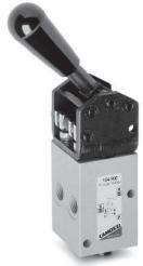
Series 3 manual valves (G1/8) and Series 4 (G1/4), 3/2 - 5/2-way and 5/3way, are available with several devices designed to satisfy different needs. The 3/2-way valves Series 3 and 4 are normally closed when 1 is the inlet; they can also be normally open when 3 is the inlet. Series 3 and 4 5/2-way valves can be supplied via the ports 3 and 5 with two different pressures, if a cylinder has to be operated using a delivery pressure which is different from the return pressure.
