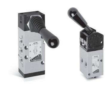
Series 3 manual valves (G1/8) and Series 4 (G1/4), 3/2 - 5/2-way and 5/3way, are available with several devices designed to satisfy different needs. The 3/2-way valves Series 3 and 4 are normally closed when 1 is the inlet; they can also be normally open when 3 is the inlet.
