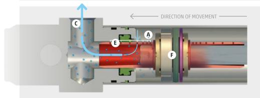
As the piston **(F)** moves, the holes **(E)** close off one by one causing a consequential decrease in the air flow from the chamber **(A)** towards the outlet **(C)**, generating a progressive and smooth deceleration.
