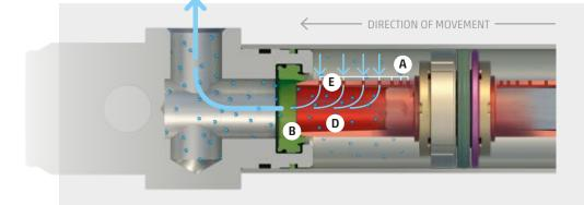
When the sleeve (**D**) reaches the seal (**B**), the air present in the chamber (**A**) is forced to pass through the holes (**E**) in the sleeve, causing the start of the slowdown.
