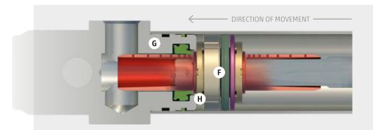
The movement stops when the end stroke position is reached and the piston (F) touches the end block (G). The presence of a damper (H) absorbs any residual kinetic energy and minimises the impact so that there is no vibration or noise.
