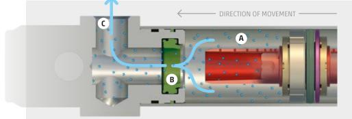
During the free movement phase, the air contained in the chamber (A) passes through the seal (B) and is exhausted through the outlet (C).
